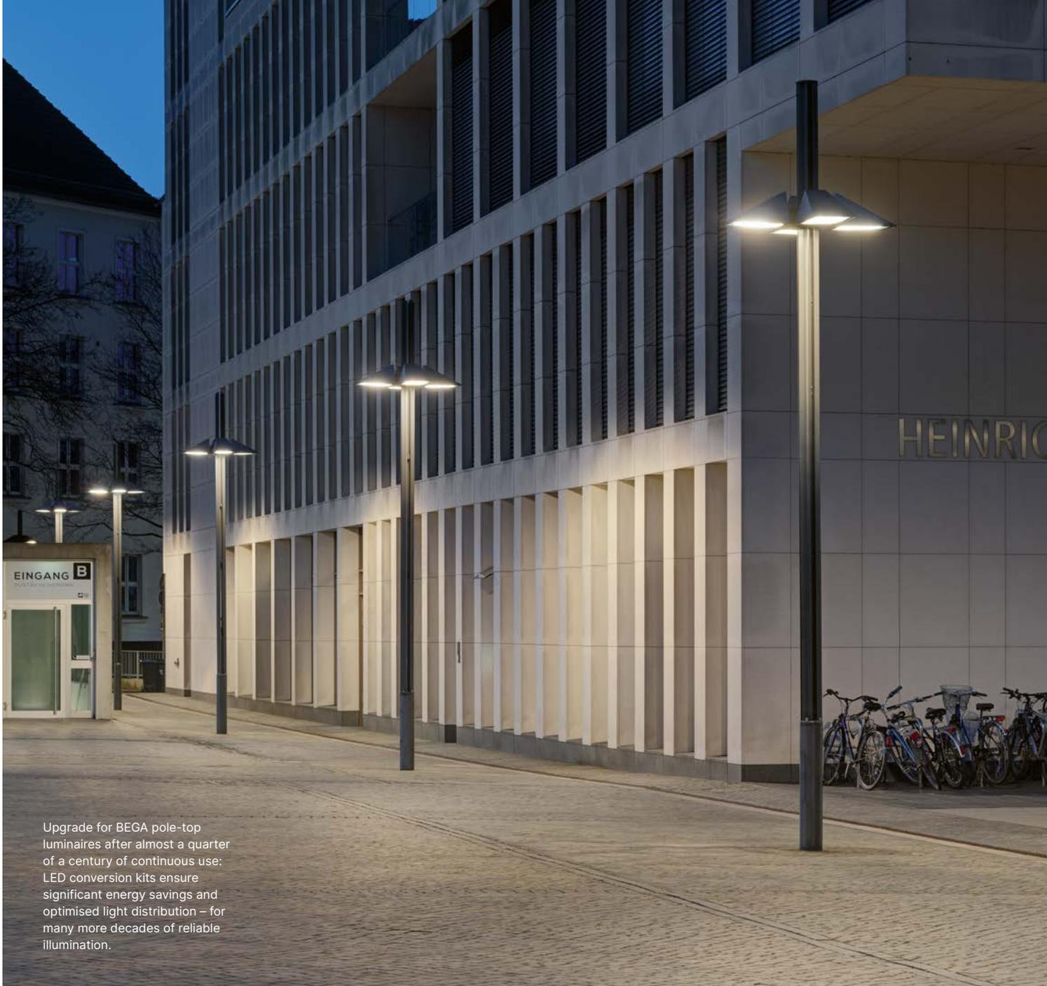
Upgrade for BEGA pole-top luminaires after almost a quarter of a century of continuous use: LED conversion kits ensure significant energy savings and optimised light distribution – for many more decades of reliable illumination.
